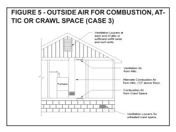
As an alternative to creating an opening in the floor to draw air from a crawl space, a duct may be dropped from the attic terminating 12" above the floor.
