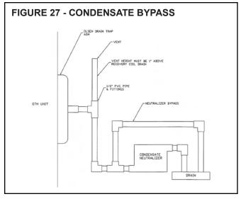
The condensate drainage configuration requires a vent. It takes less than a one inch rise anywhere along the horizontal route of the drain tube to create a vapor lock, which will prevent condensate from draining away freely, and result in erratic furnace operation.
