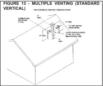
If more than two furnaces are being installed in close proximity, each additional combustion air intake and exhaust termination set shall not terminate less than 12 in (300 mm) apart. Note: Canadian installations of 120000 Btuh require 3 ft (900 mm).
