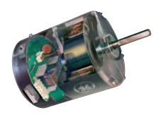
**ECM (Electronically Commutated Motor) = Lower operating costs.** At full load the ECM motor is 20% more efficient than a conventional motor. On continuous fan speed, the ECM motor consumes 60-80 watts compared to 400 watts for a conventional motor.
