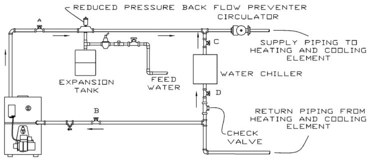
Figure 7 Bypass Piping Typically Used With Baseboard Heating
