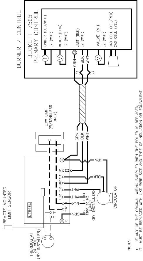
WHEN LOW LIMIT IS USED, SET "ELL" PARAMETER ON L7248L CONTROL TO ON. BOILERS FACTORY EQUIPPED WITH TANKLESS COIL ARE FACTORY SET TO ON.
