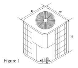
The dimensions for the condensing unit are illustrated in Figure 1. Physical and electrical specifications are provided in Table 1 for 13 SEER systems respectively.
