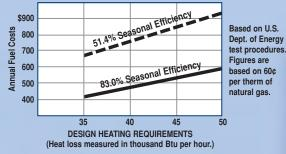
This graph illustrates the difference in annual operating costs between boilers with higher and lower efficiencies. Boilers installed ten or more years ago have seasonal efficiencies as low as 50%. So, your savings in fuel dollars with Olsen's ODV-B boiler can repay its installed cost in a few short years!
