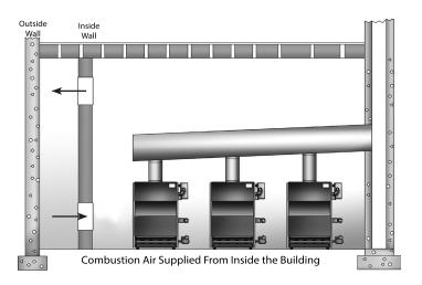
Figure 9 - Combustion Air with Motorized Dampers
